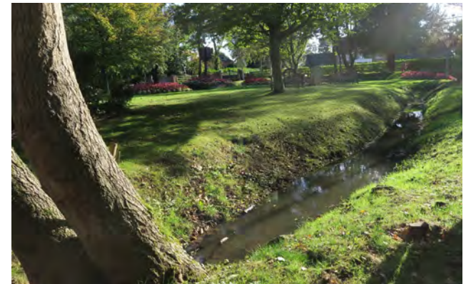
Figure 44: A network of swales takes the water north and then west in stages until it discharges into the Trinity Broads.
